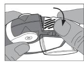
Close the side chamber door and dispose of the used strip.
